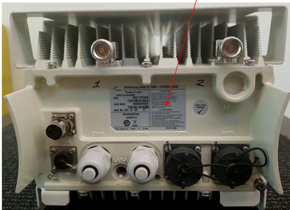
“AirHarmony 4200 3550-3700MHz (B48)” side panel, label with FCC ID:PIDAH4200 location
