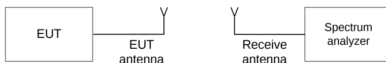
Figure 7.3.1 Occupied bandwidth test setup
