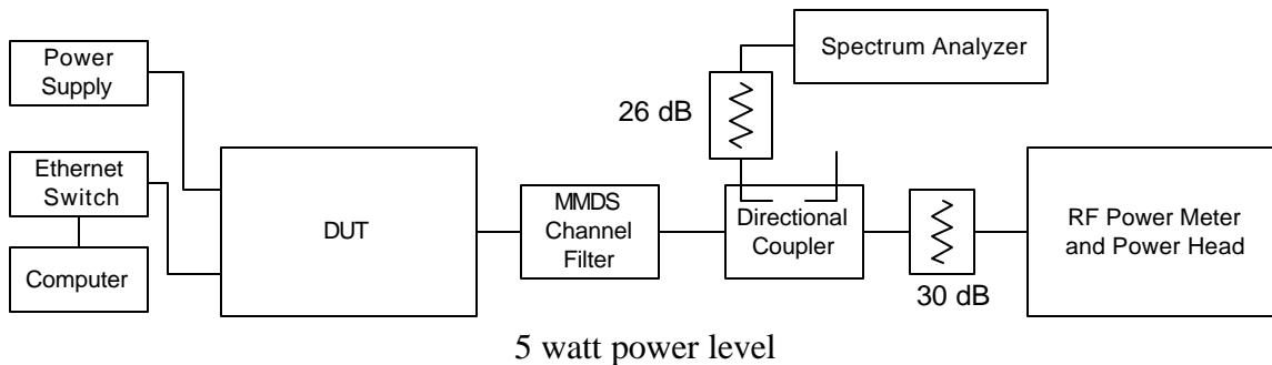
Test Results: 100 % transmit duty cycle
