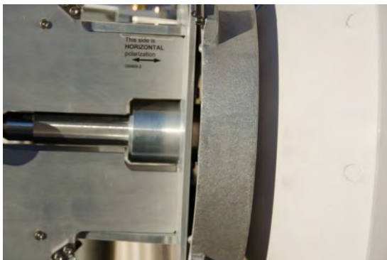
Figure 6-3: Dual Pole Adapter Polarization Label
