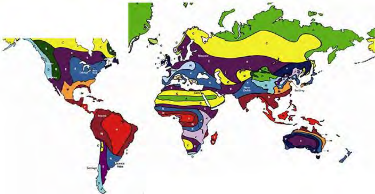
Figure 2-3: ITU rain zone chart of the earth
