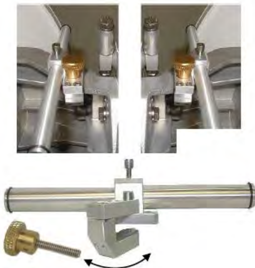
Figure 5-13: Re-configuring Alignment Sight Tool
