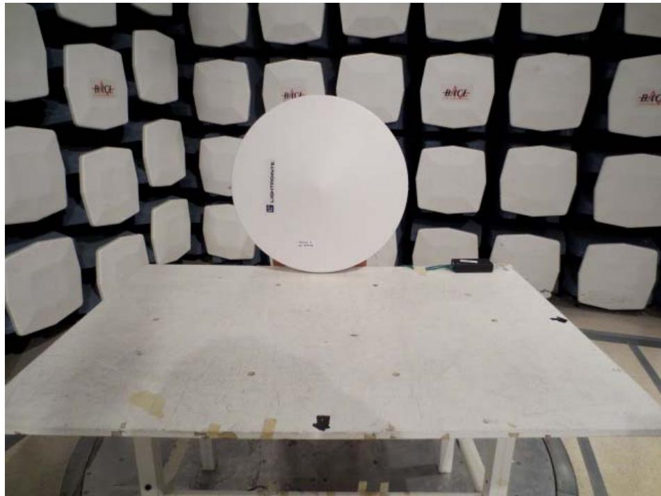
**9.8 Above 1 GHz Spurious Radiated Emissions (EUT with 1 ft. Antenna) – Rear View**
