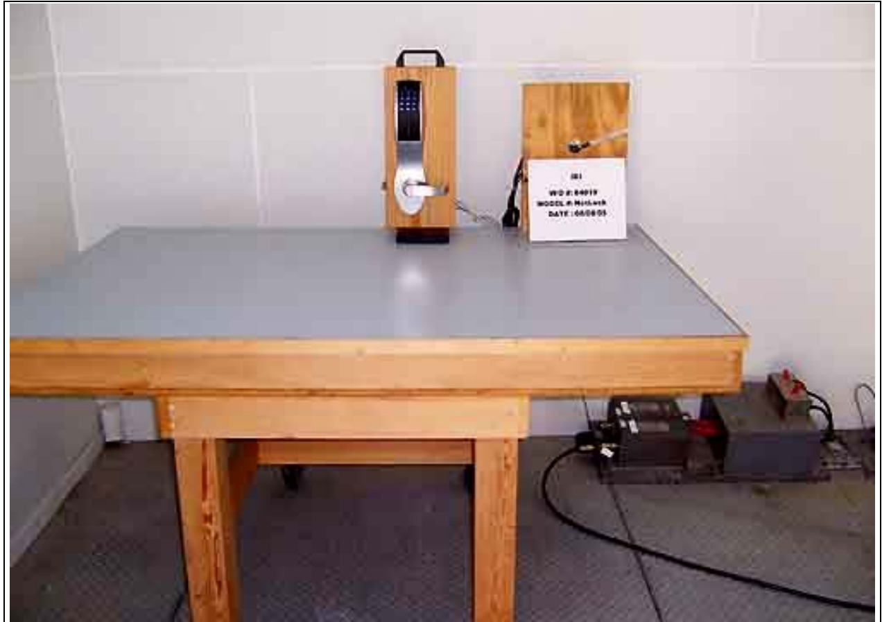
Mains Conducted Emissions - Front View
