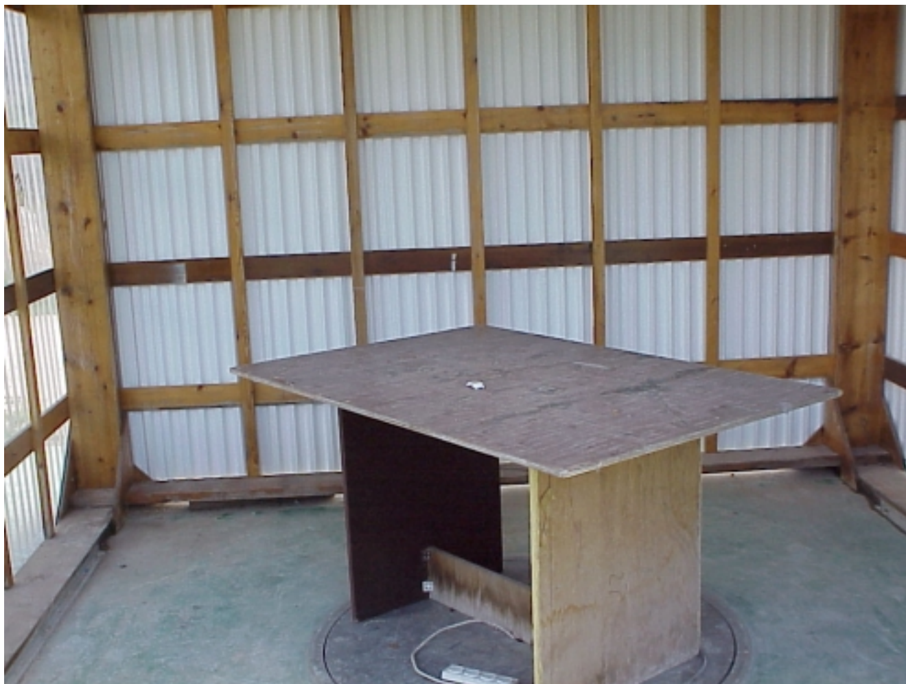
Photo#1. Radiated emissions measurements on the open site
