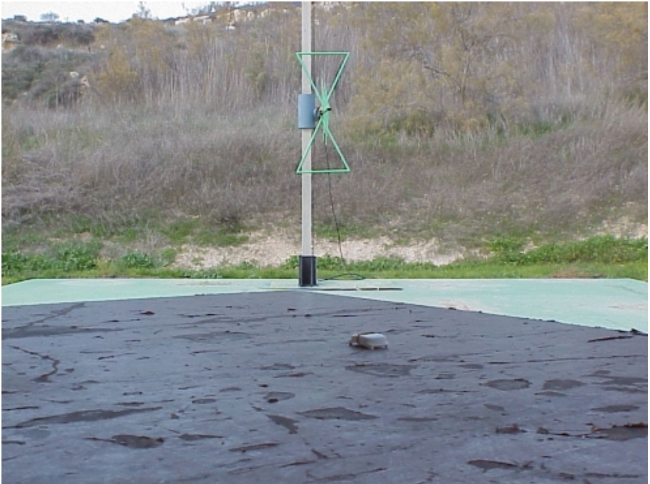
Photo#3 Radiated emissions measurements on the open site
