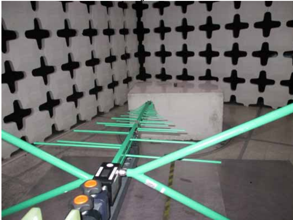
Test Setup for Radiated Emissions – 30MHz to 1GHz, Horizontal Polarization, Ventis Pro 4
