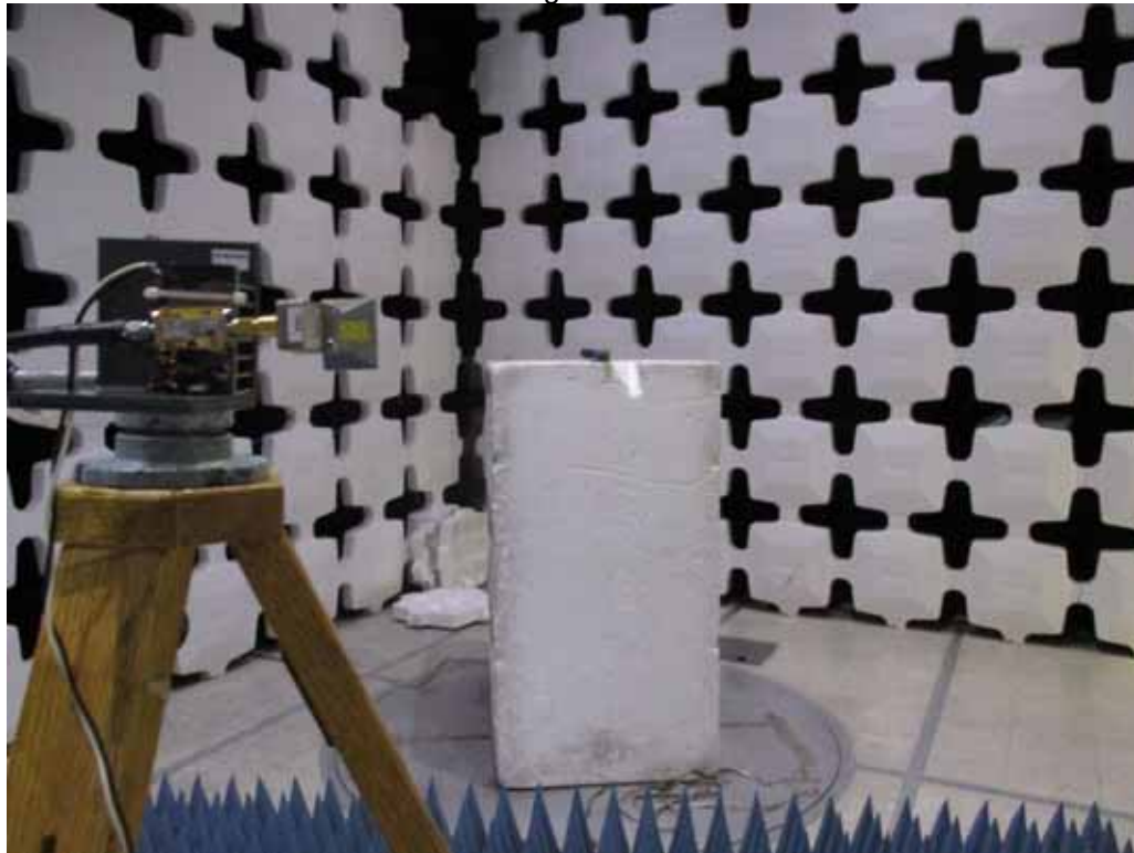
Test Setup for Radiated Emissions – 18GHz to 25GHz, Horizontal Polarization, Ventis Pro 4
