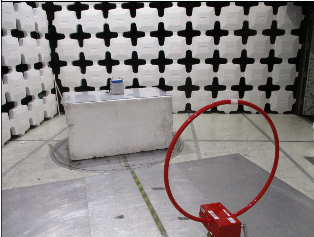
Test Setup for Spurious Radiated Emissions, 10-30MHz – Antenna Polarization Vertical
