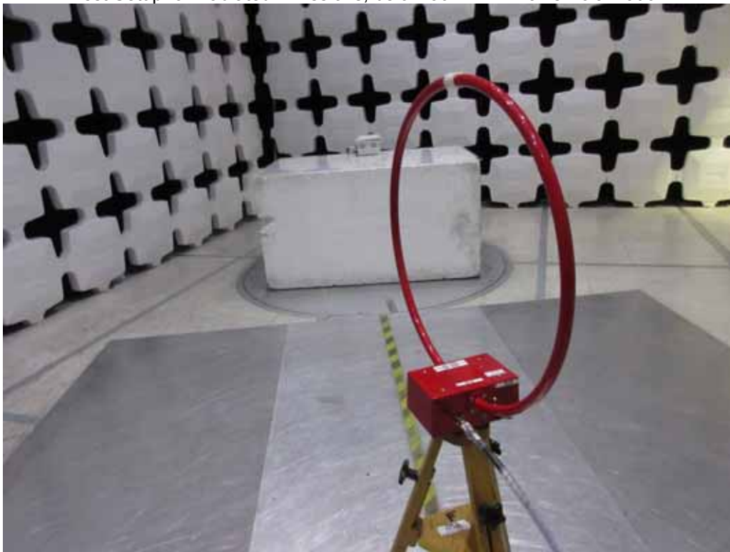
Test Setup for Radiated Emissions, below 30MHz – Y axis Polarization
