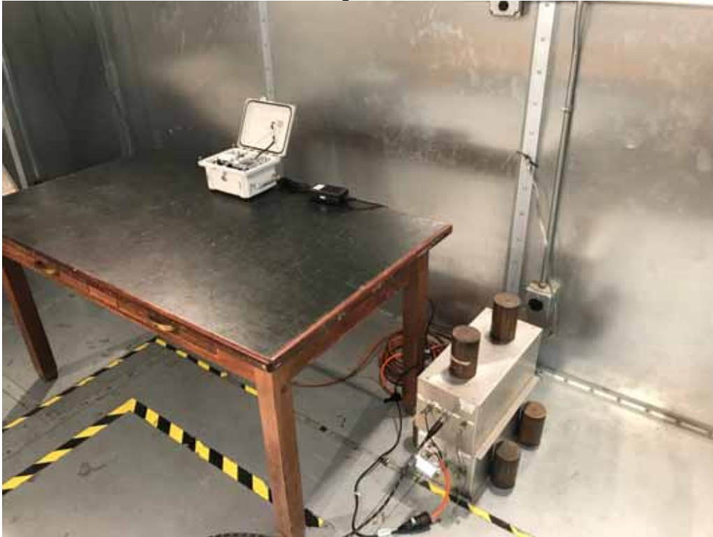
Test Setup for Conducted Emissions
