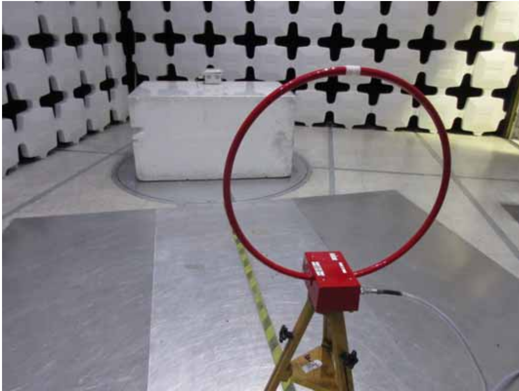
Test Setup for Radiated Emissions, below 30MHz – X axis Polarization
