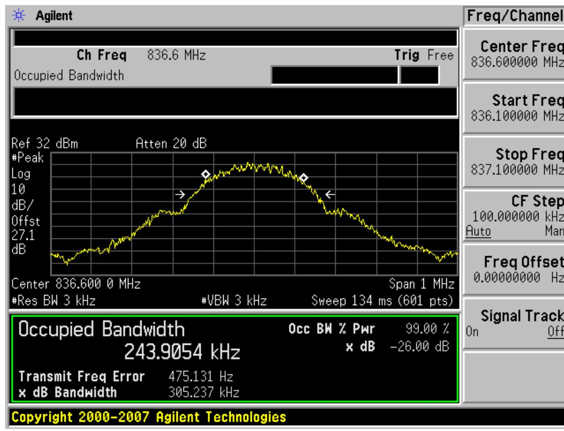
■ GSM850 MODE (251 CH.) Occupied Bandwidth
