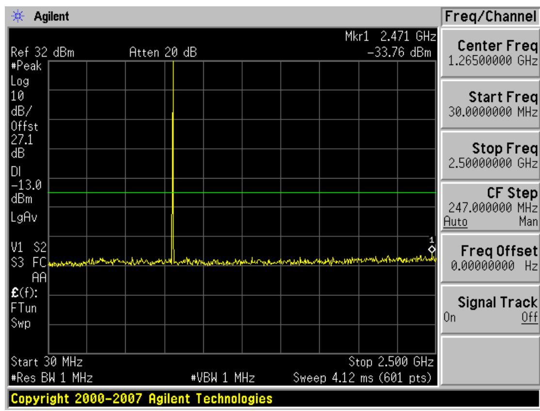
■ GSM850 MODE (128 CH.) Conducted Spurious Emissions2
