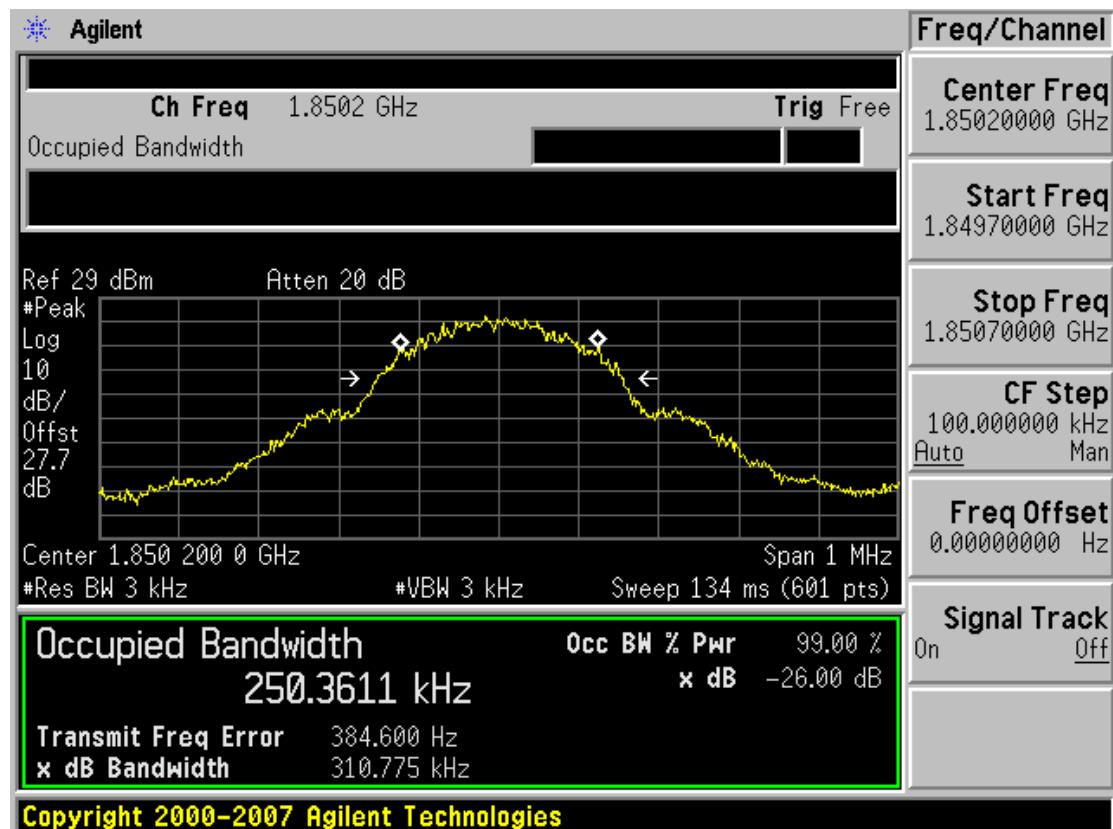
■ GSM1900 MODE (661 CH.) Occupied Bandwidth
