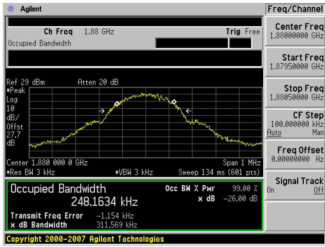
■ GSM1900 MODE (810 CH.) Occupied Bandwidth
