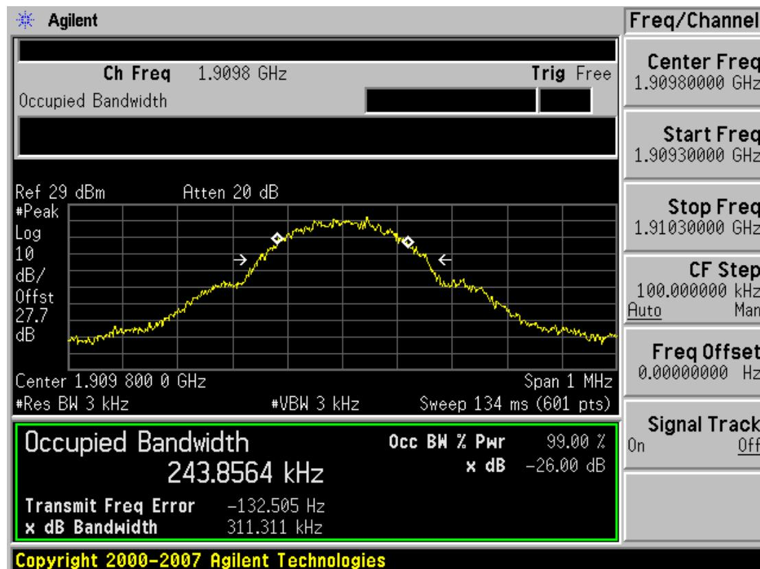
■ GSM1900 EDGE (512 CH.) Occupied Bandwidth
