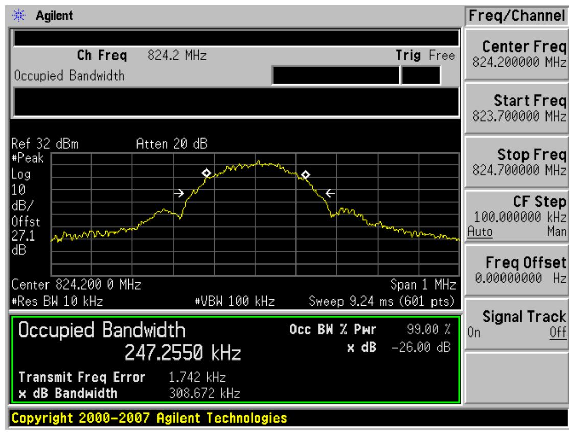
■ GSM1900 MODE (512 CH.) Occupied Bandwidth
