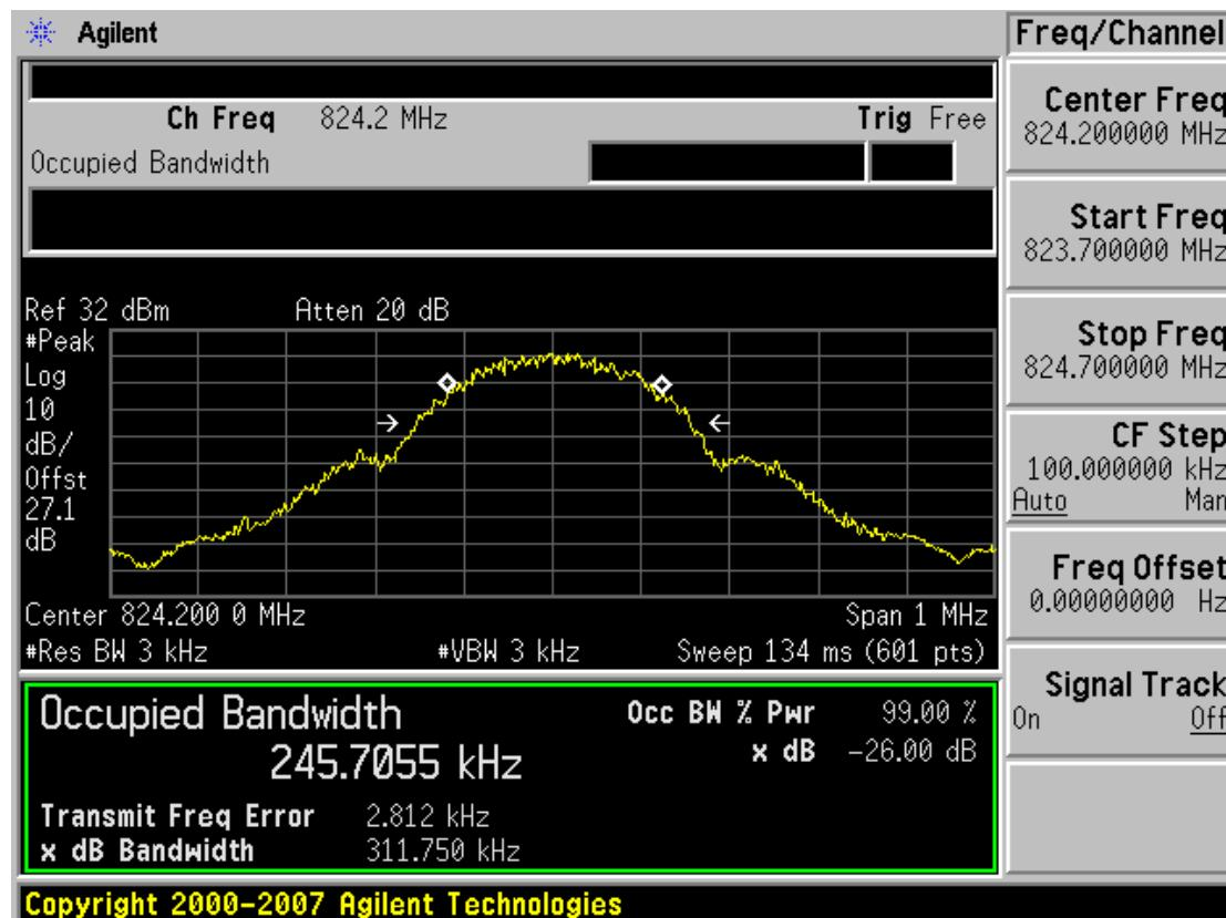
■ GSM850 MODE (190 CH.) Occupied Bandwidth
