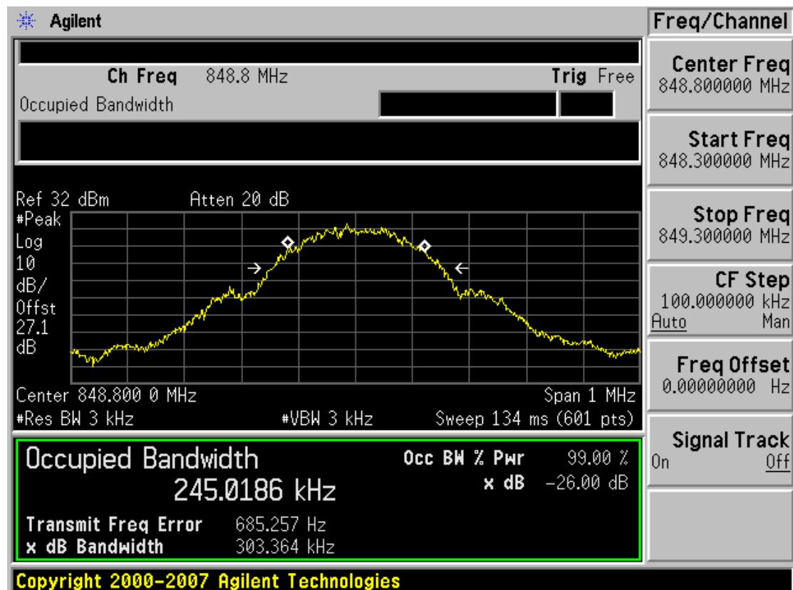
■ GSM850 EDGE (128 CH.) Occupied Bandwidth
