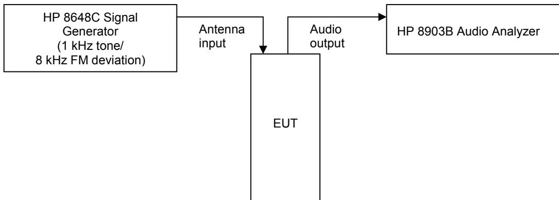
Frequencies used on the signal generator were 824.04, 836.50, and 848.97 MHz for the mobile band, and 869.04, 881.50, and 893.97 MHz for the base band.
