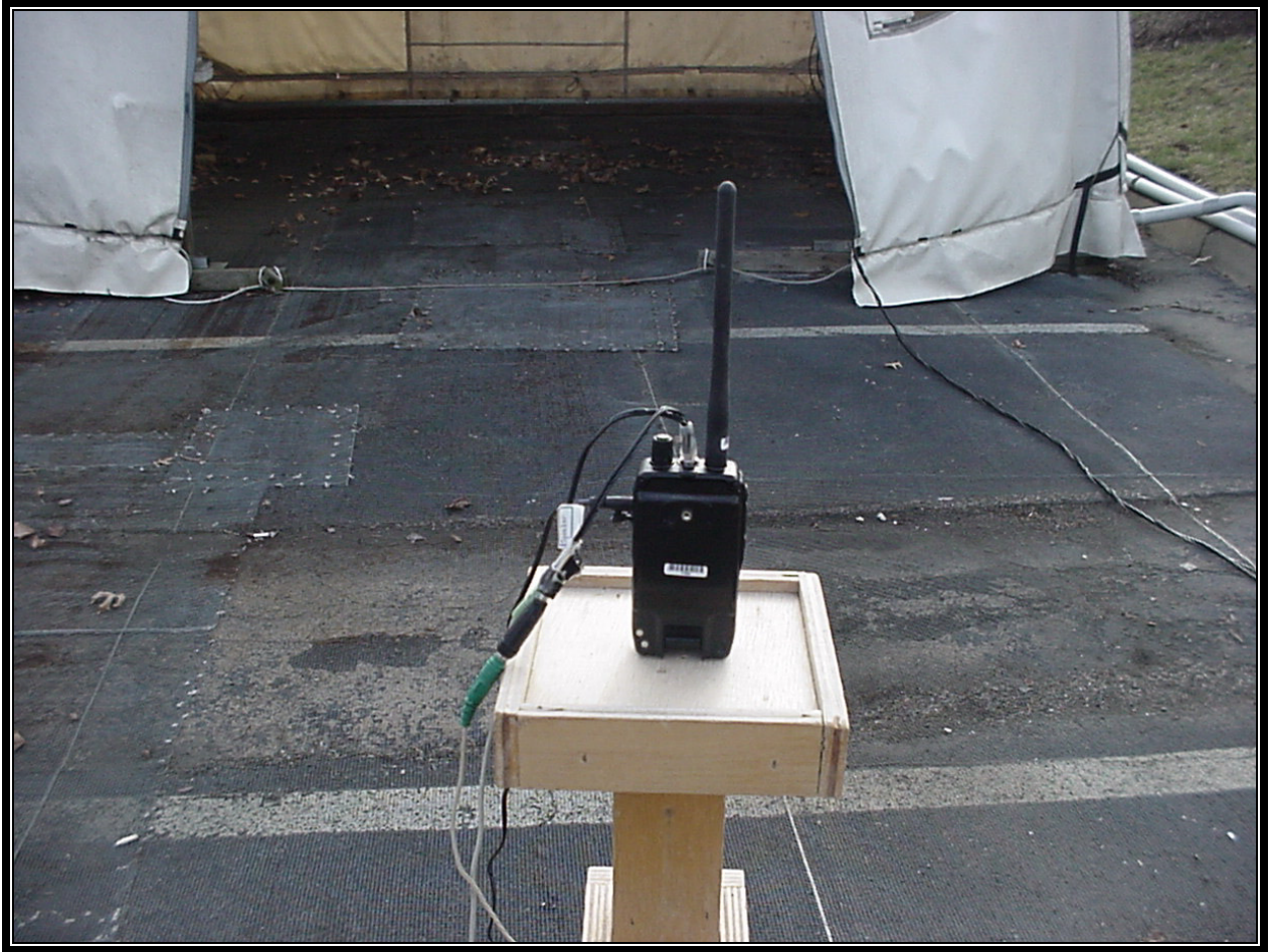
Photograph 4: Radiated Emissions Test Configuration (Rear View)
