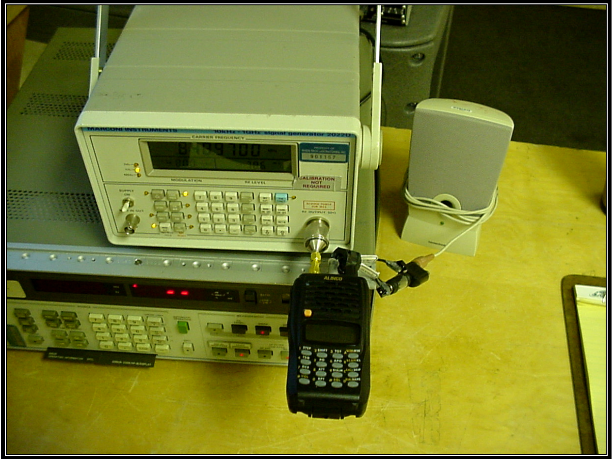
Photograph 5: 38 dB Rejection Test Configuration
