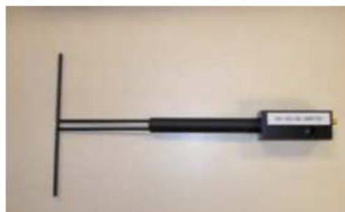
Figure 1 – Satimo COMOSAR Validation Dipole
