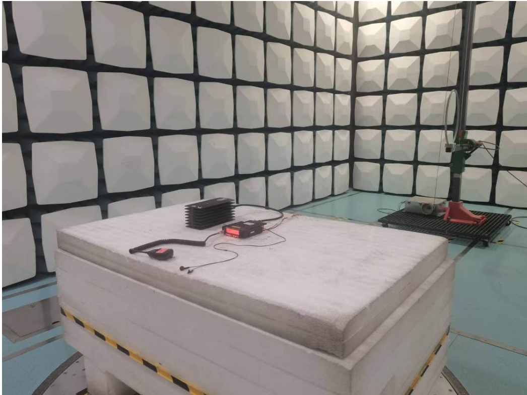
Radiated Emission 9k-30MHz Perpendicular View
