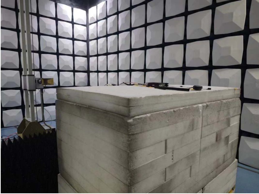
Radiated Emission 18-25GHz View
