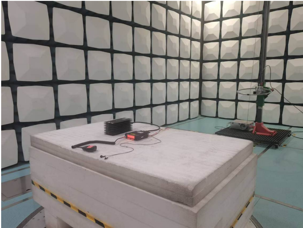
Radiated Emission 30M-1GHz View
