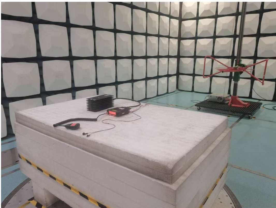
Radiated Emission 30M-1GHz View
