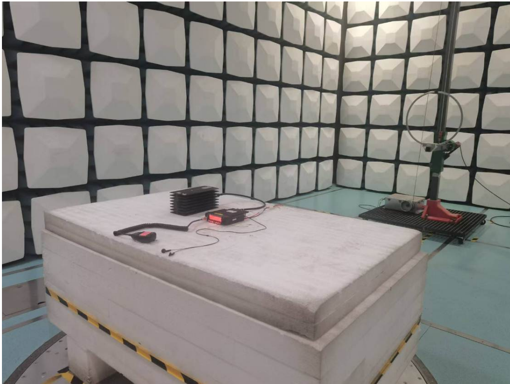
Radiated Emission 9k-30MHz Perpendicular View
