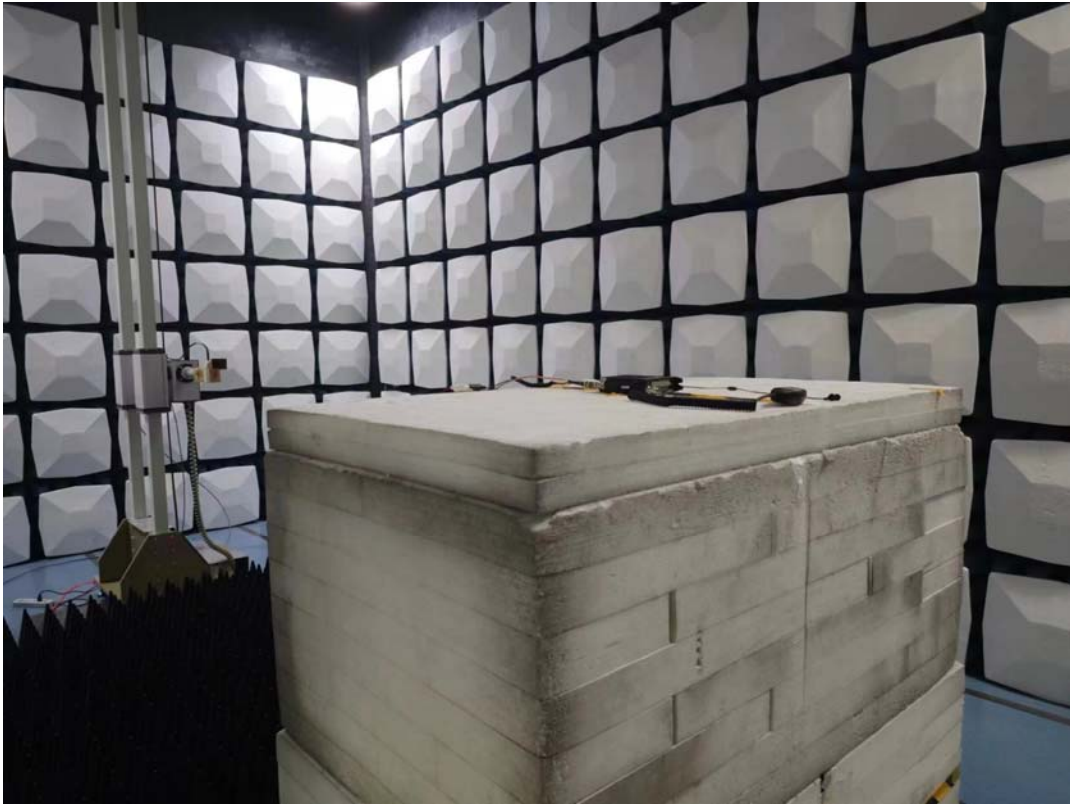
Radiated Emission 18-25GHz View
