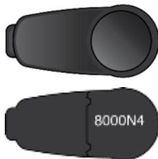
The transmitter snaps into the transmitter holder and wirelessly sends your glucose information to your display device(s).
