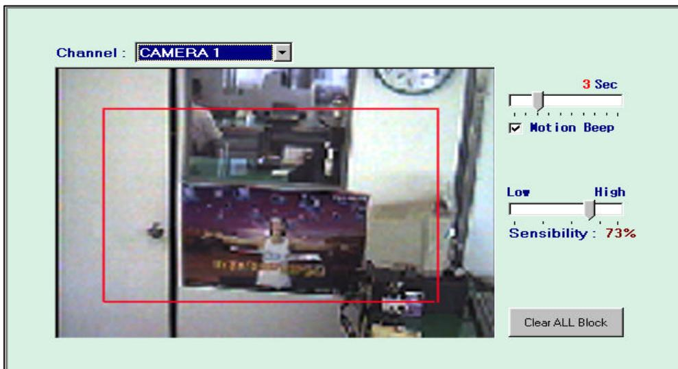
Set up motion detection zone. It would be seen in red square (Maximum 10 areas per camera).
