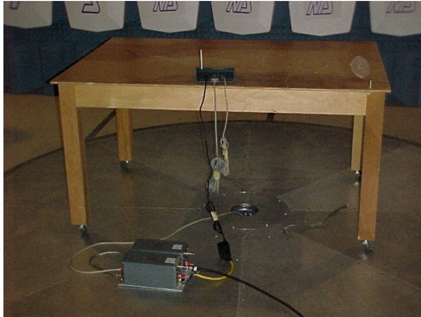
Conducted Test Setup for AC Power line
