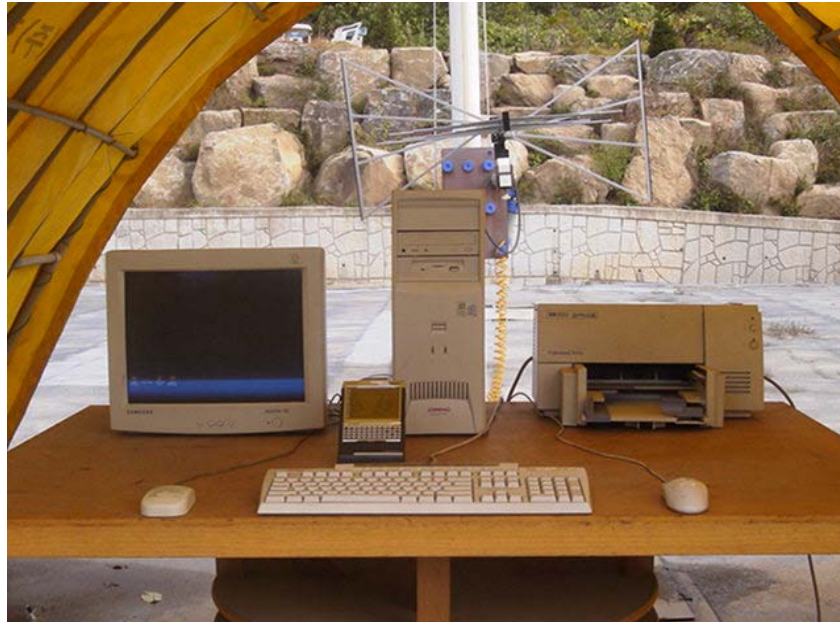
Photograph 1 : Setup for radiated Emissions
