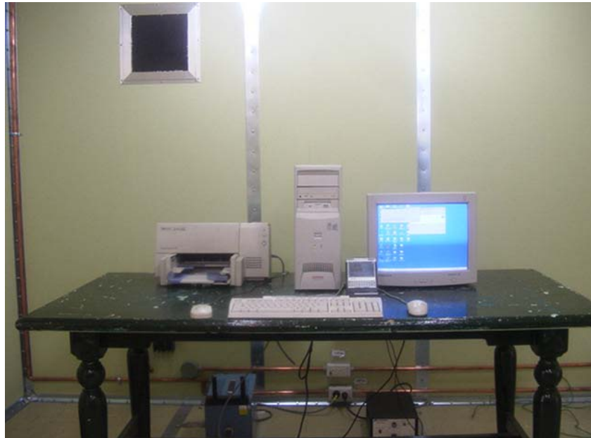
Photograph 2 : Setup for Conducted Emissions
