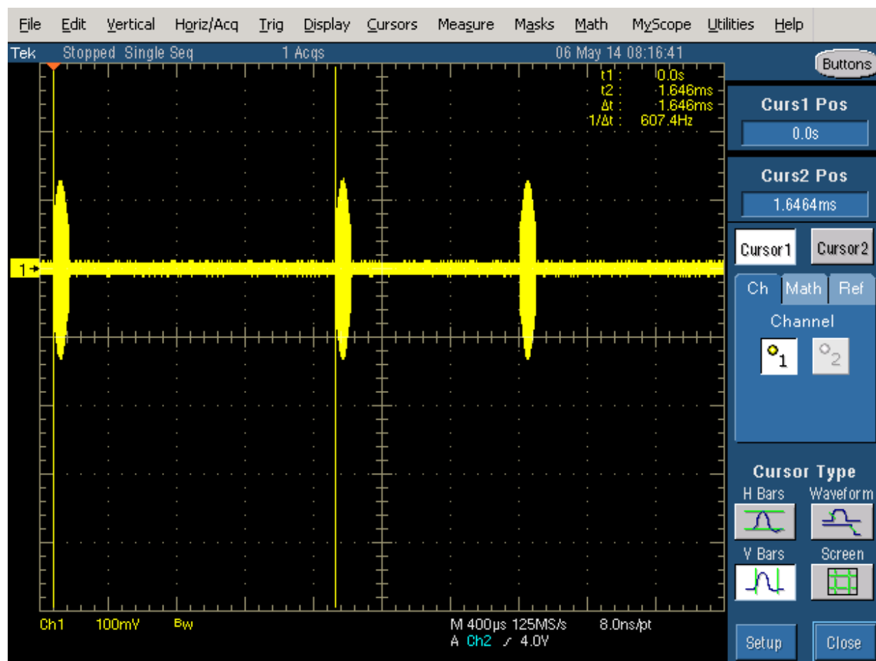
Figure 6 FCC Type 5 Radar (burst with three pulses, 1650 μs first period)
