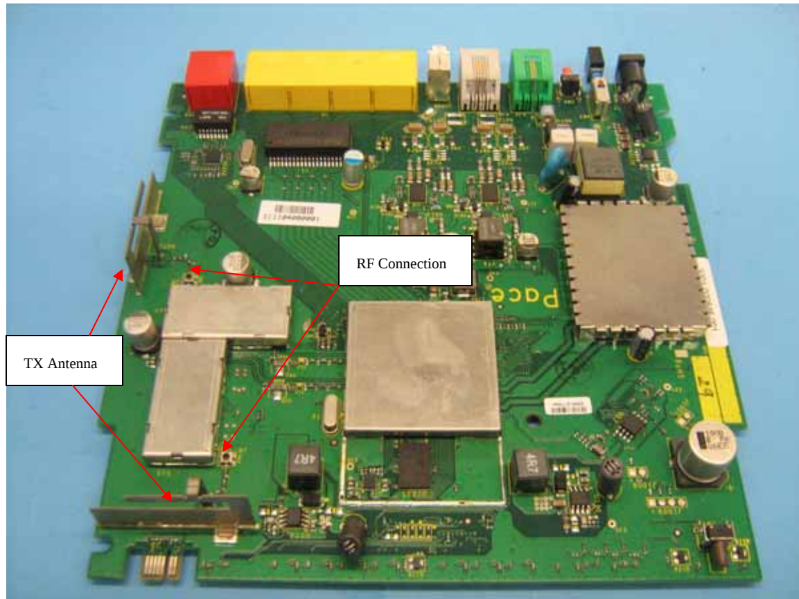
Figure 1: Internal Photo of 5111NV - PCB Board (Front Side)
