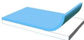
**Adhesive:** Cross-linked, long life, acrylic, pressure-sensitive adhesive, typified by a medium tack, a very high shear and temperature performance.
