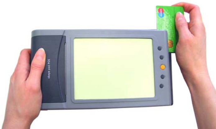
Fig. 12: Reading a magnetic card
