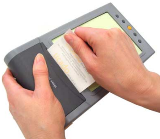
Fig. 15: Tearing paper along the paper cutter; step 1
