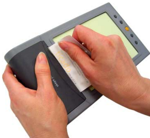
Fig. 16: Tearing paper along the paper cutter; step 2
