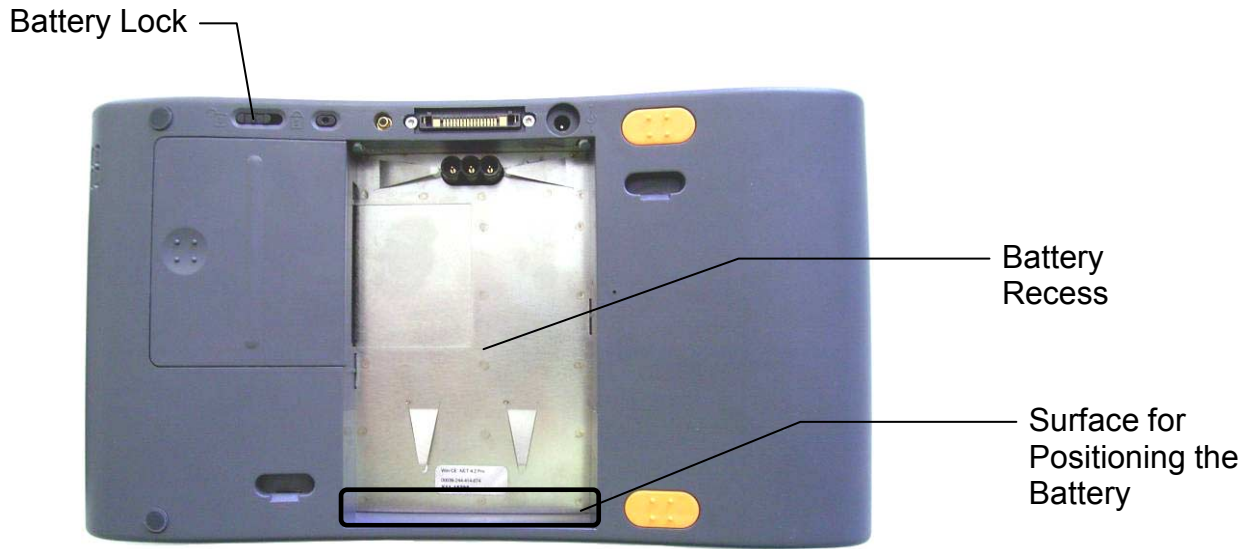
Fig. 24: Rear view of skeye.pad POS with battery removed
