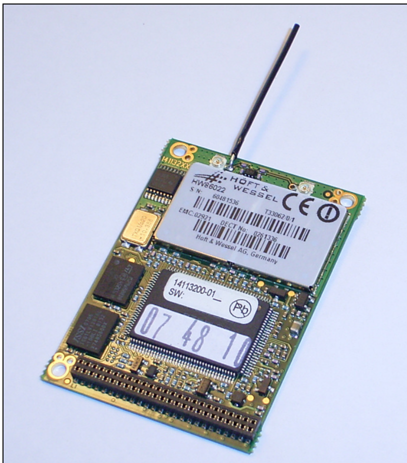
Figure 10: HW 86022 with wire antenna mounted on ANT1 port.
