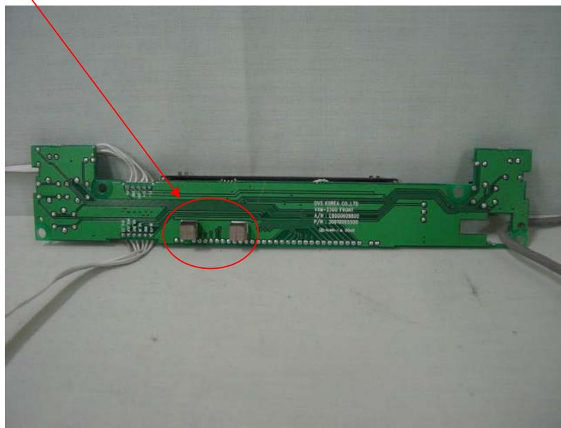
3. Attach a **finger** on the AV interface Board
