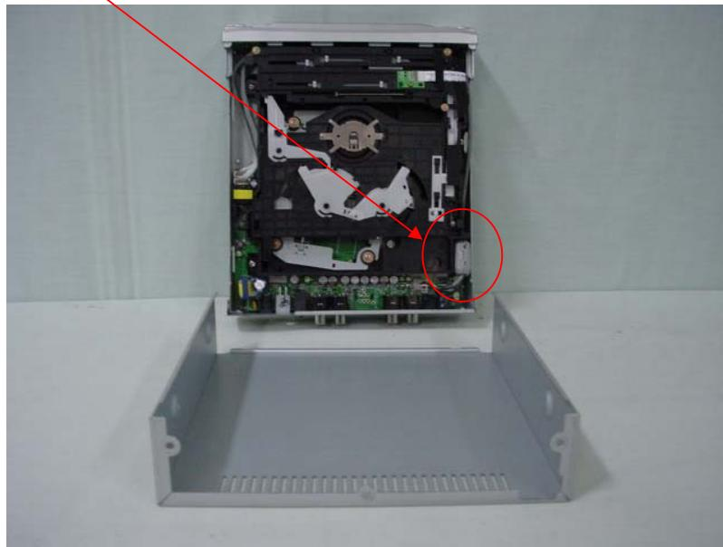
2. Attach a **gasket** on the front board
