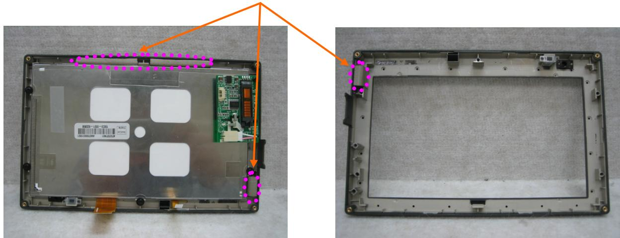
**2. Attach a gasket on the Board**
