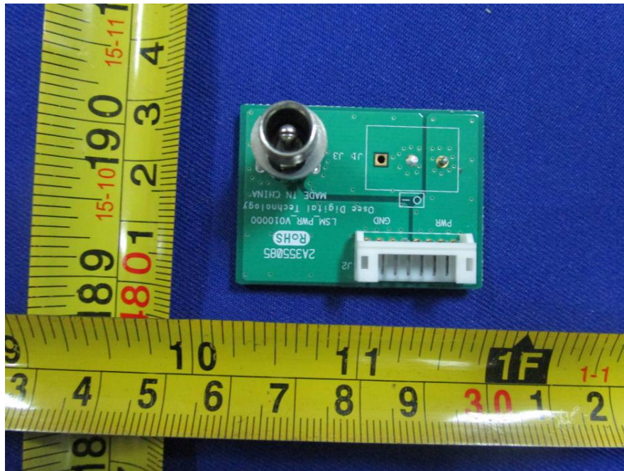
EUT –Power Board Top View
