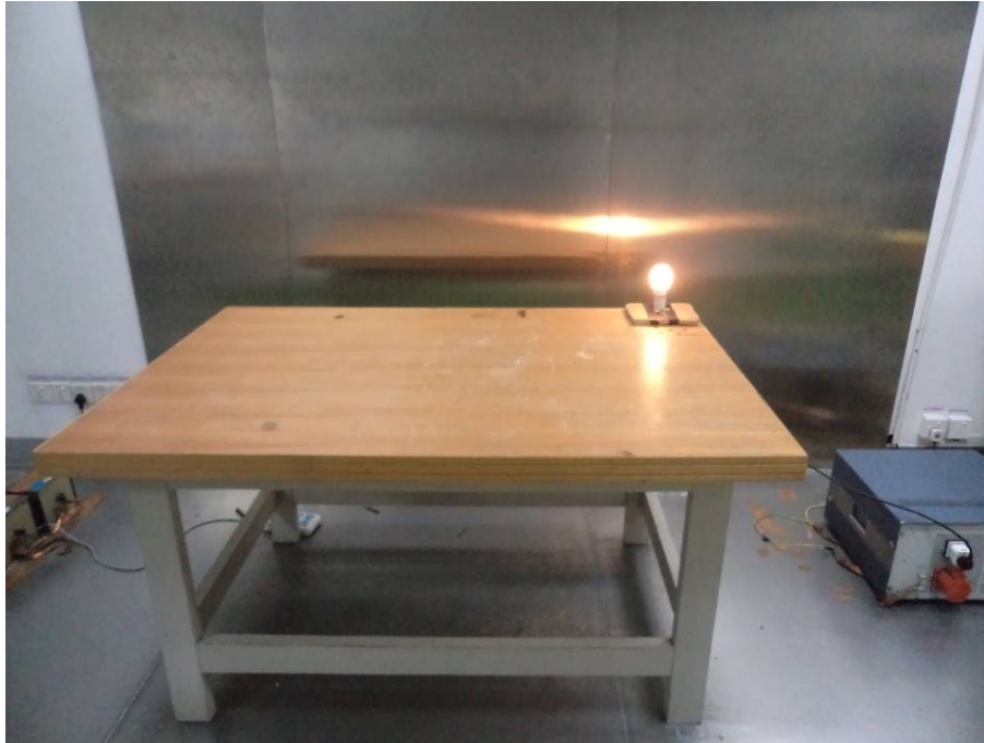
AC Line Conduction Emissions – Front View
