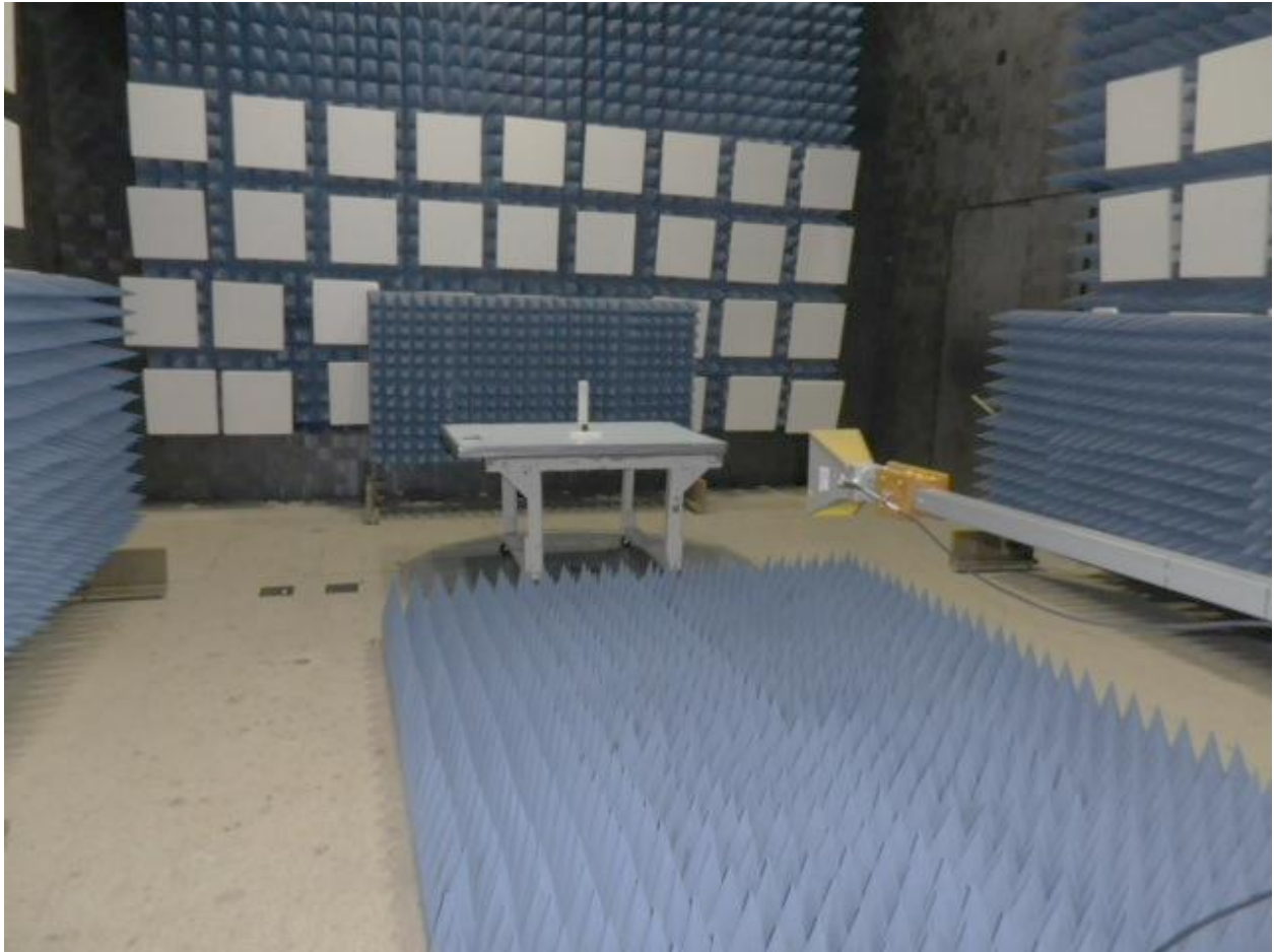
Figure 3: Typical Radiated Emissions – Above 1 GHz shown, Front view
