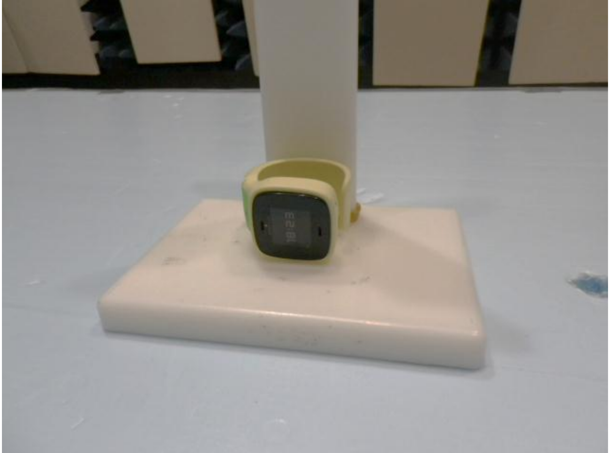
Figure 8: Radiated Emissions – Orientation C Investigation for highest emissions
