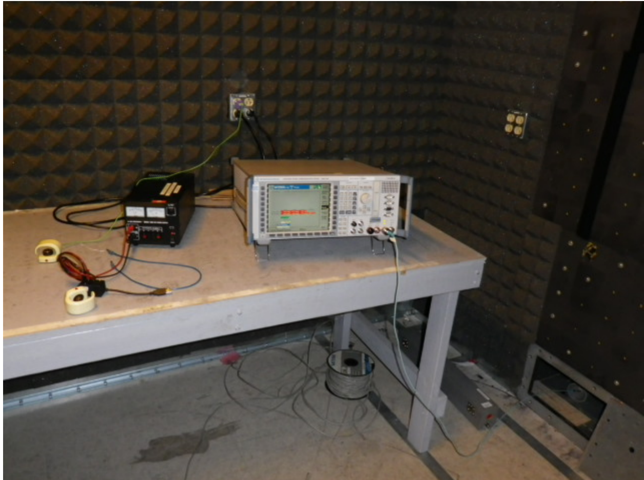
Figure 5: Network Simulator in Ancillary Chamber
