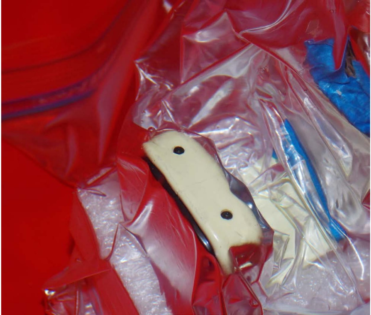
Device Set in Tissue For Extremity Testing
