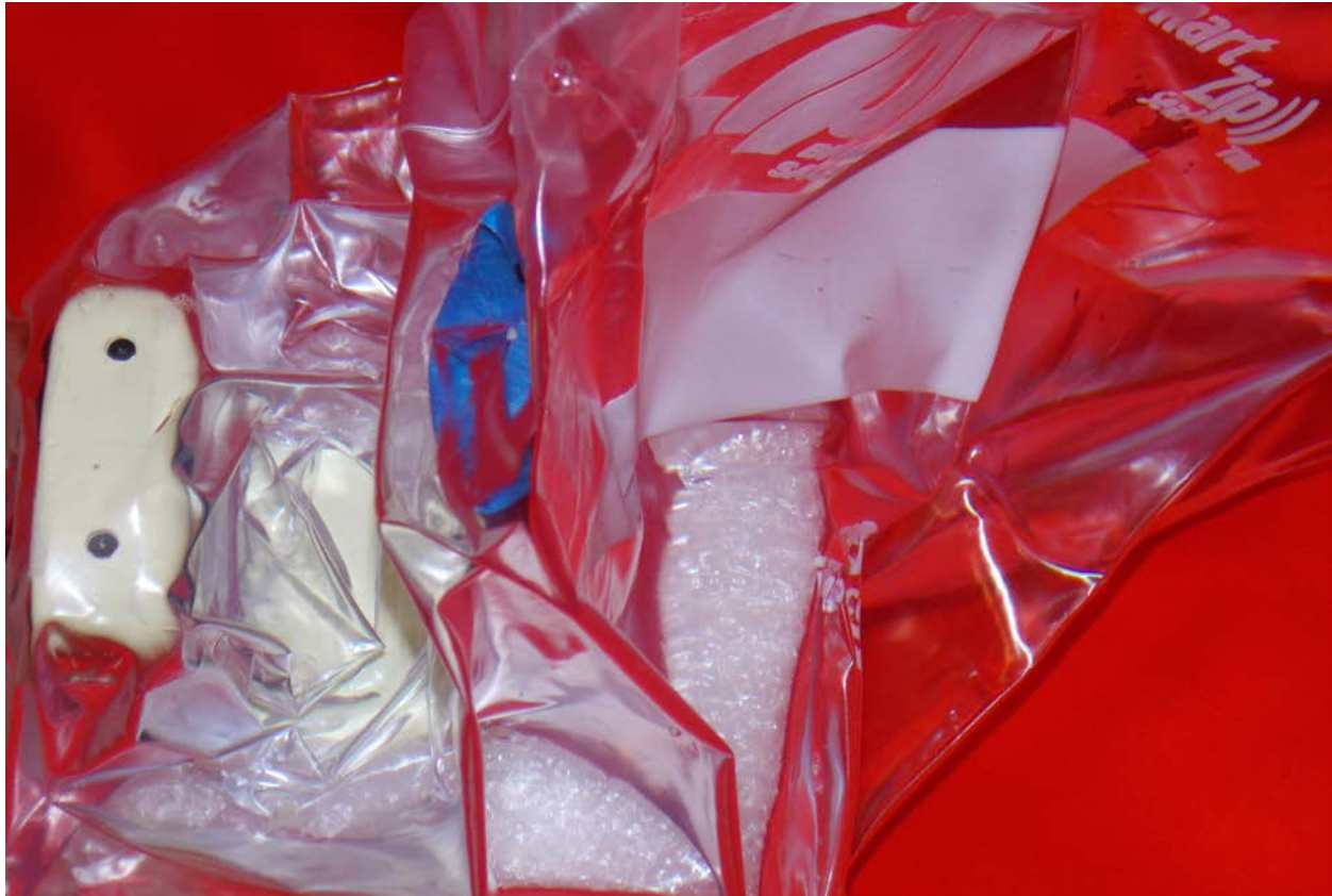
Device Set in Tissue For Extremity Testing
