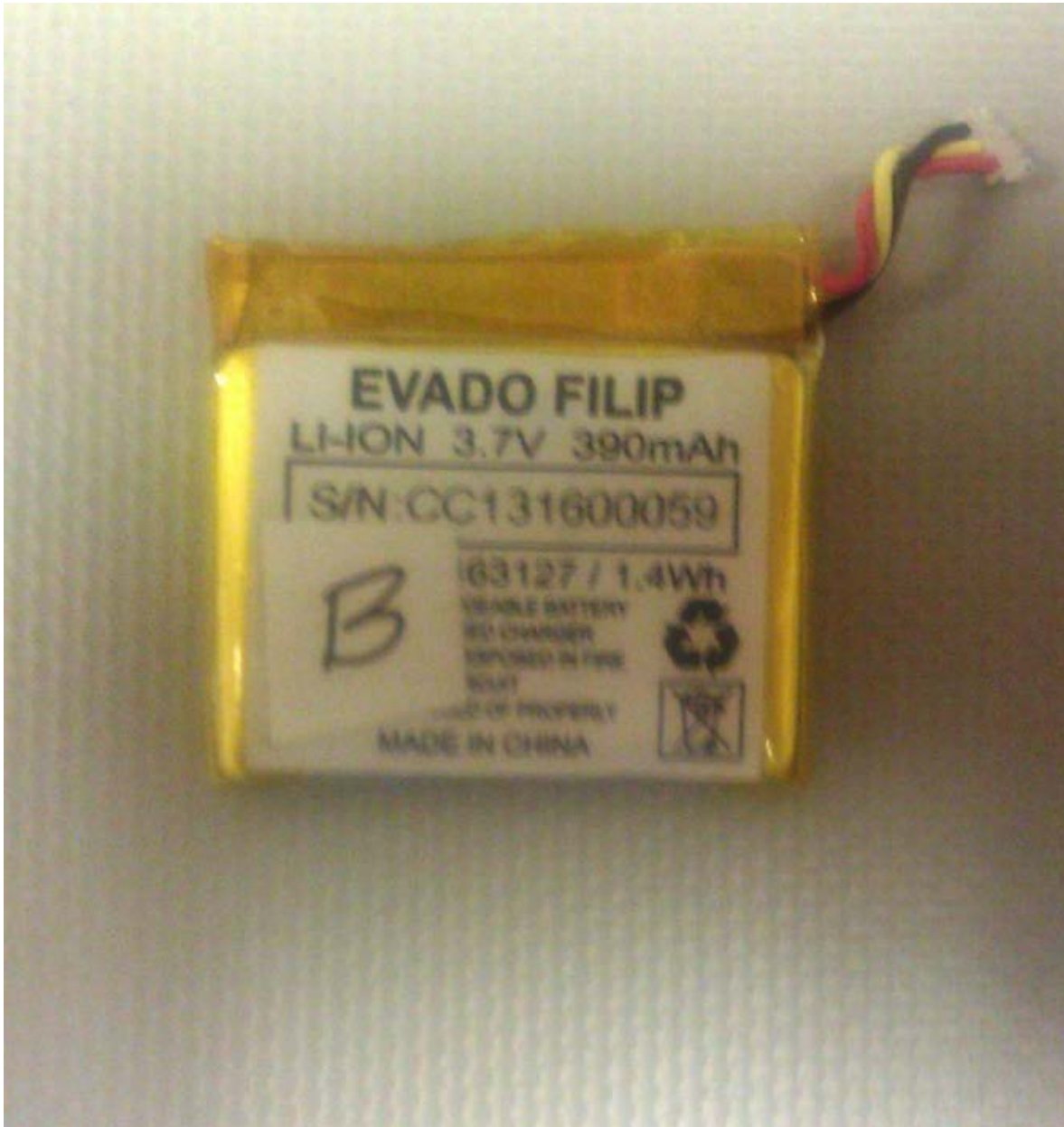
Figure 7: Internal View of EUT – Battery assembly
