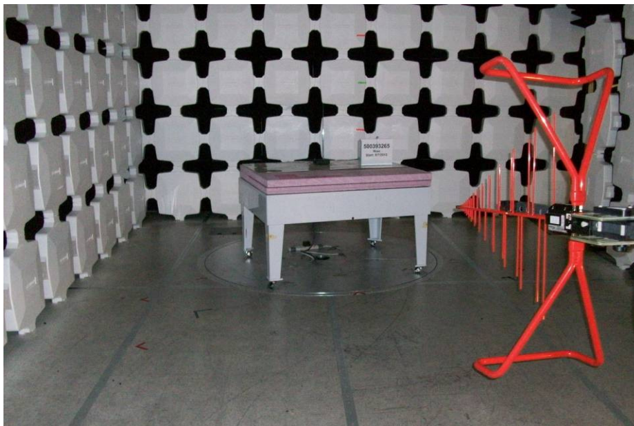
Antenna Setup: BiLog Antenna – 30MHz to 1000MHz
