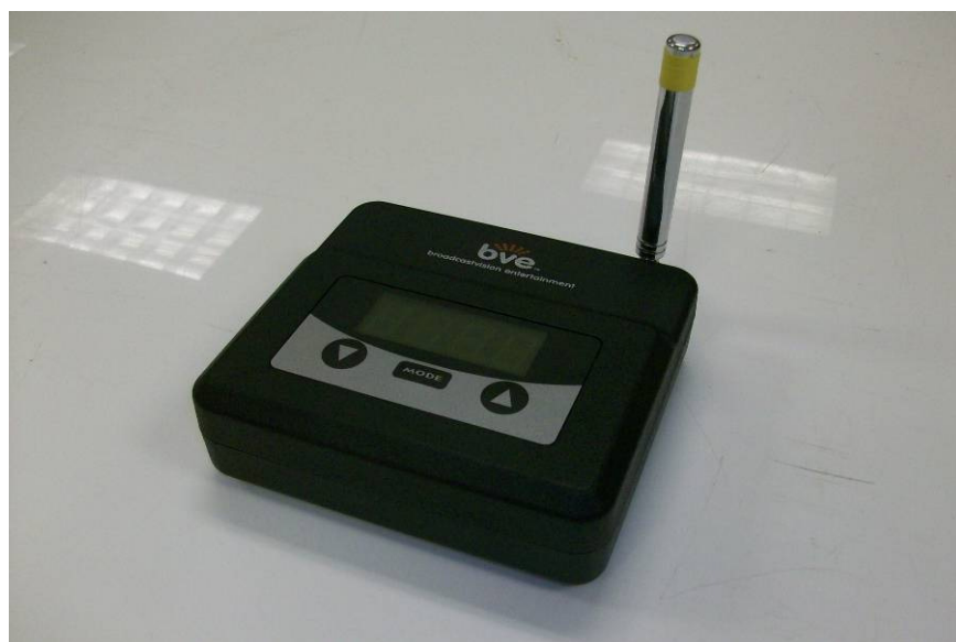
Shown with antenna fully retracted – 900MHz operation
