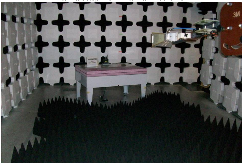
Antenna Setup: Horn Antenna – Above 1GHz
