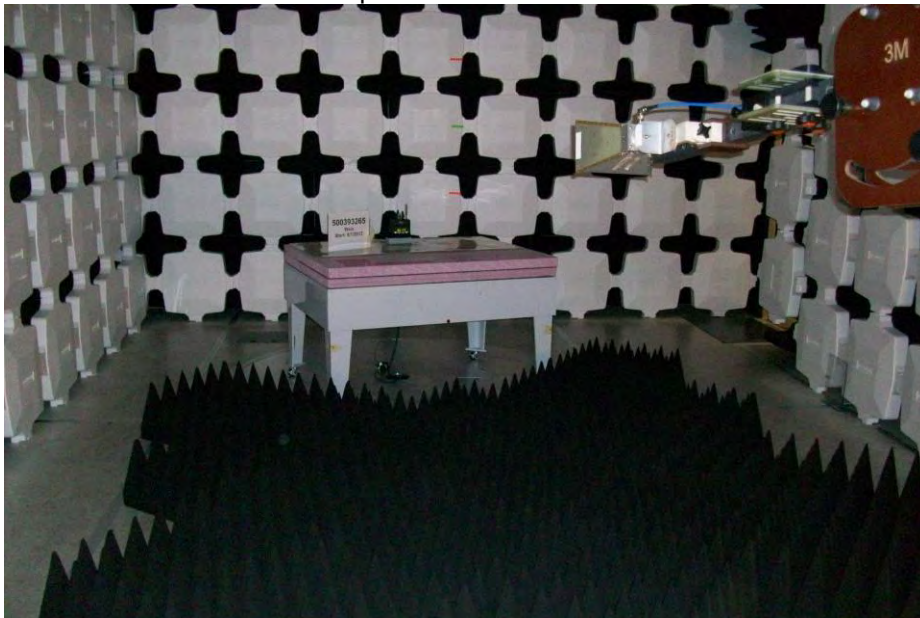
Antenna Setup: Horn Antenna – Above 1GHz
