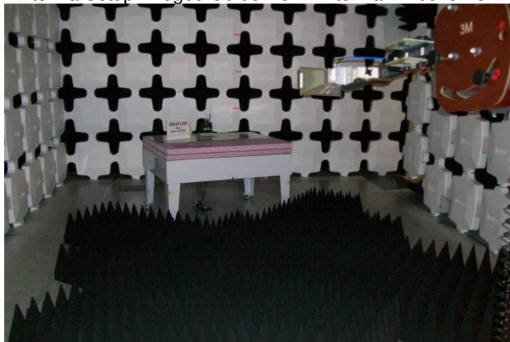
Antenna Setup: Ridged Guide Horn Antenna – Above 1GHz
