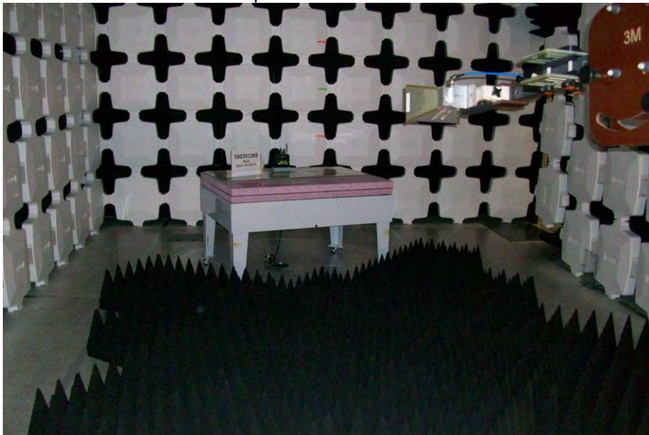
Antenna Setup: Horn Antenna – Above 1GHz
