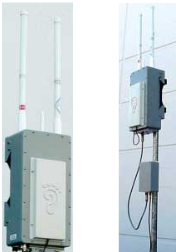
figure 32. cSPICE installed on a wall (left) and pole (right)
