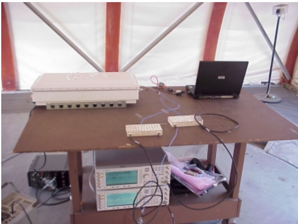
bSPICE Spurious Radiated Emissions (Rear View)
