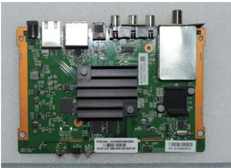
A photograph of the DMT-1434 V1.1 main board, showing its green PCB, components, and heat sinks. The board appears similar to the V1.0 version but with some internal changes. It is placed on a grey surface next to a metric ruler for scale. |
