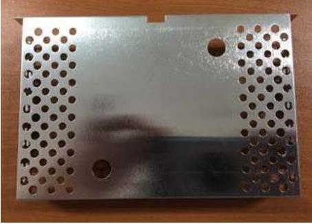
A photograph of the top shield cover for the DMT-1434 V1.1, showing a metal plate with a grid of holes and a central rectangular cutout. The design appears slightly different from the V1.0 version. |
