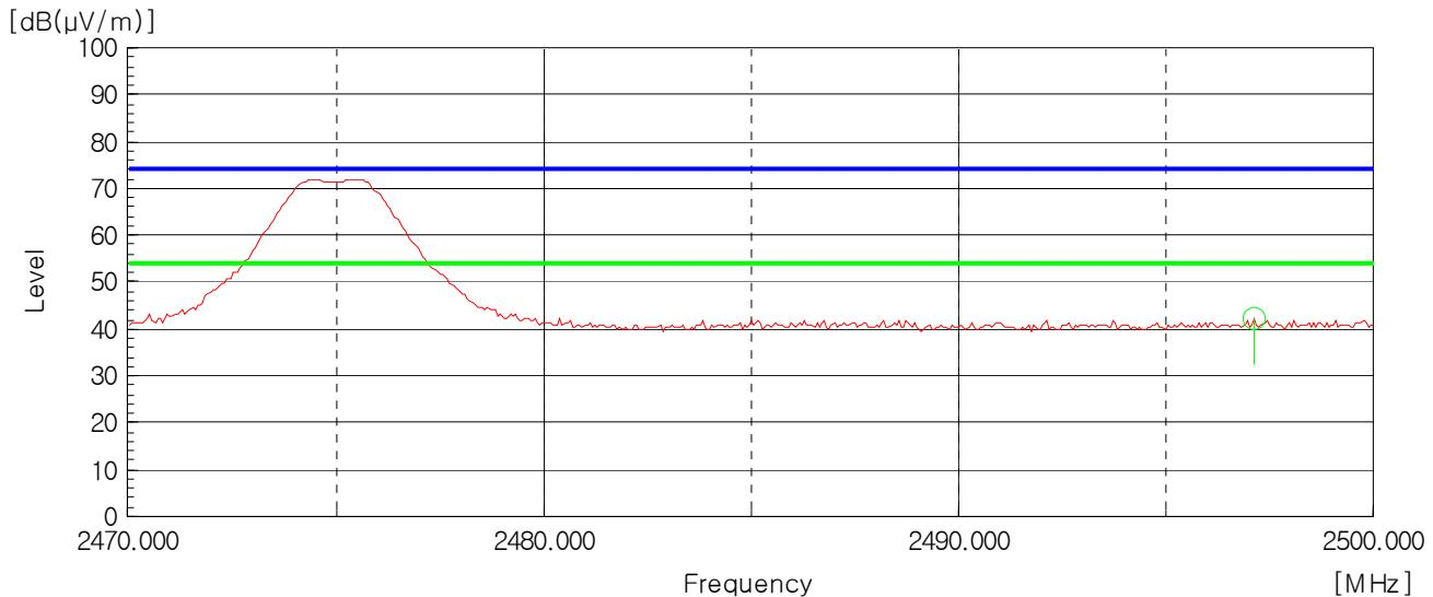
AV Detector: RBW: 1 MHz, VBW: 10 Hz (2 483.5 MHz - 2 500 MHz), Worst case (High, Horizontal)
