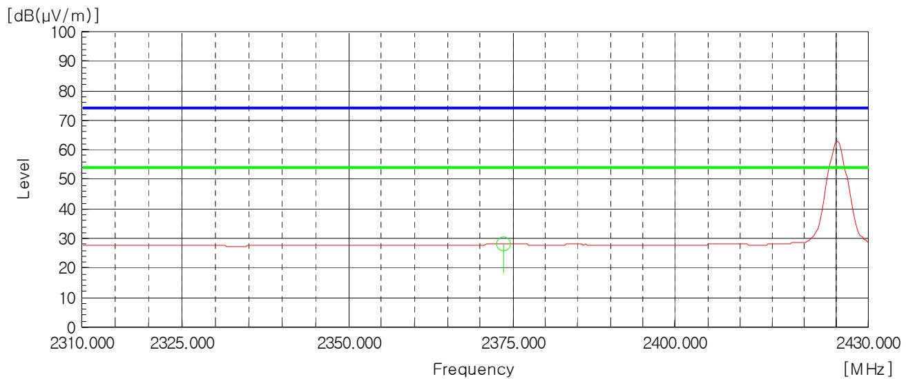
Peak Detector: RBW: 1 MHz, VBW: 1 MHz (2 483.5 MHz - 2 500 MHz), Worst case (High, Horizontal)
