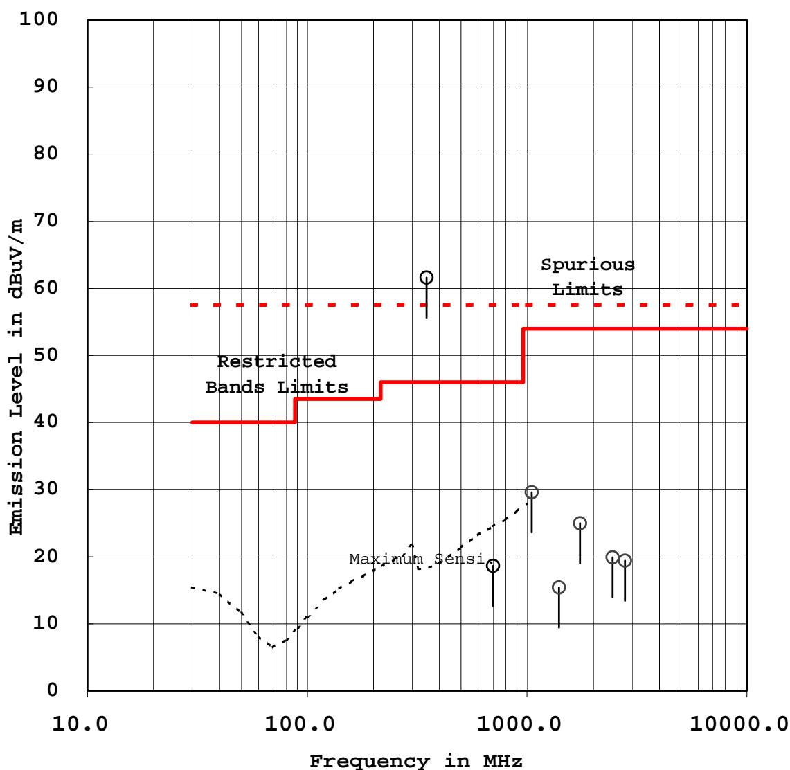
**RADIATED EMISSION MEASUREMENT**
