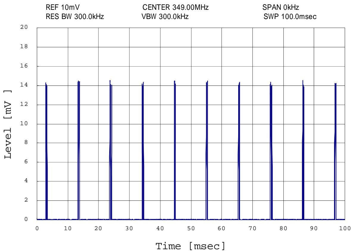
The above wave form indicates the case when field strength Average over 100ms was maximum value.
