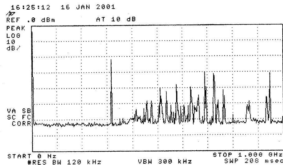
Figure 5.1. Emissions measured at 3 meters in anechoic chamber, 0-1000 MHz.
