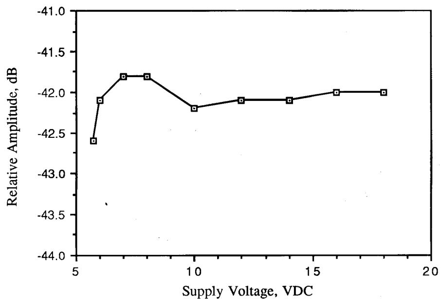
Figure 6.2. Relative emission at "fundamental" vs. supply voltage.
