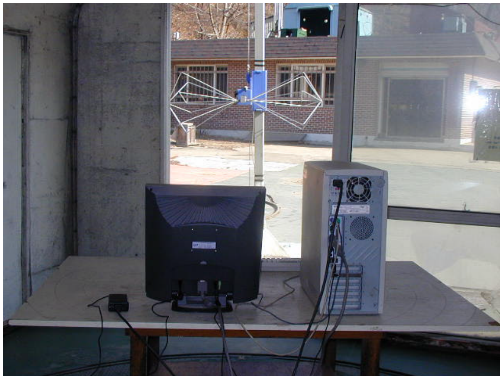
RADIATED EMISSION SETUP PHOTOGRAPH - REAR VIEW ( 30 - 300 MHz )
