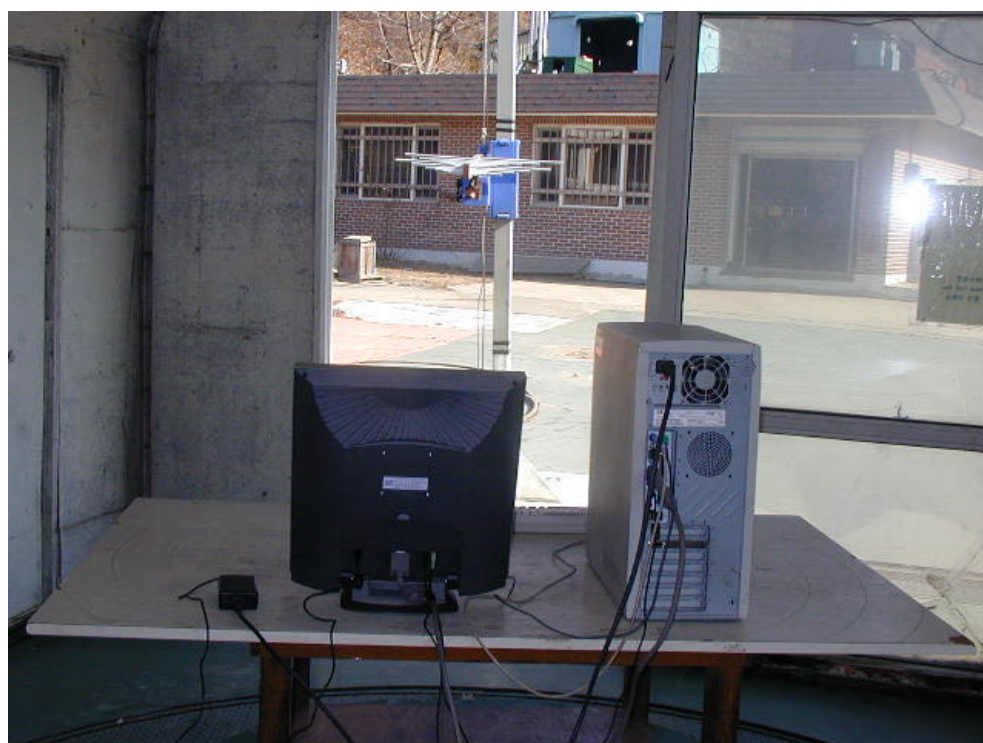
RADIATED EMISSION SETUP PHOTOGRAPH - REAR VIEW ( 300 - 1000 MHz )
