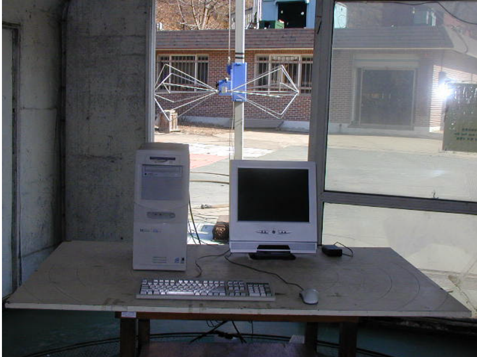
RADIATED EMISSION SETUP PHOTOGRAPH - FRONT VIEW ( 30 - 300 MHz )
