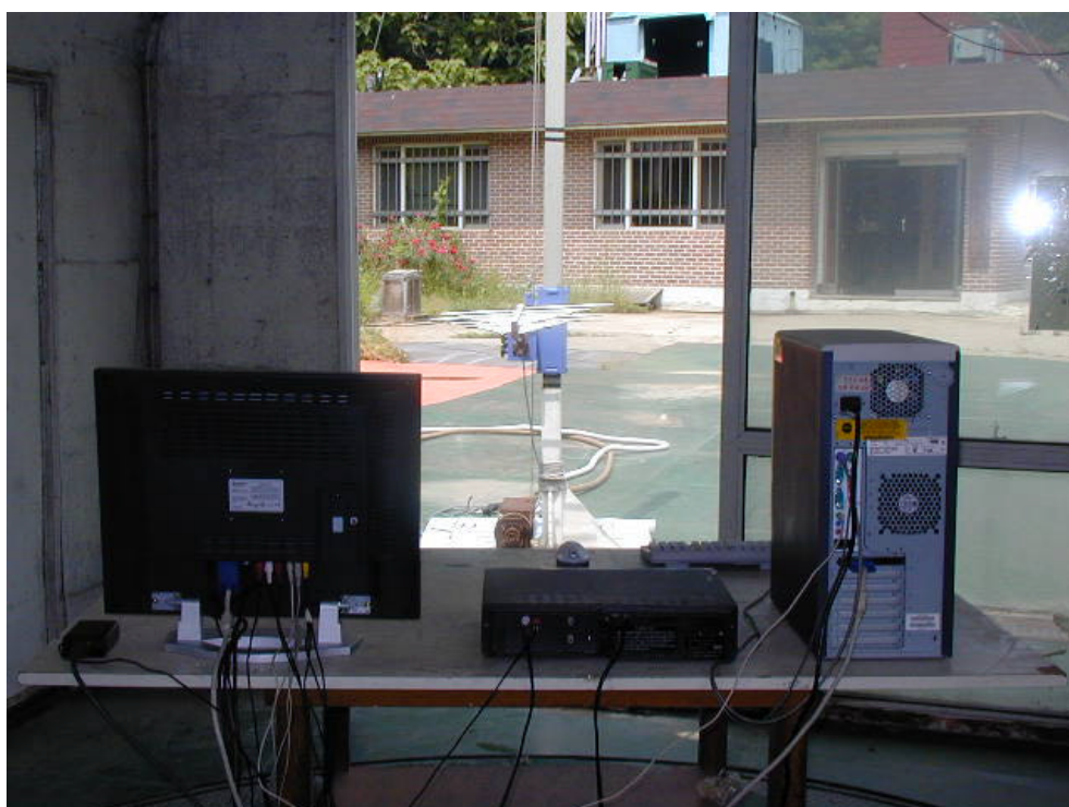
RADIATED EMISSION SETUP PHOTOGRAPH - REAR VIEW ( 300 - 1000 MHz )
