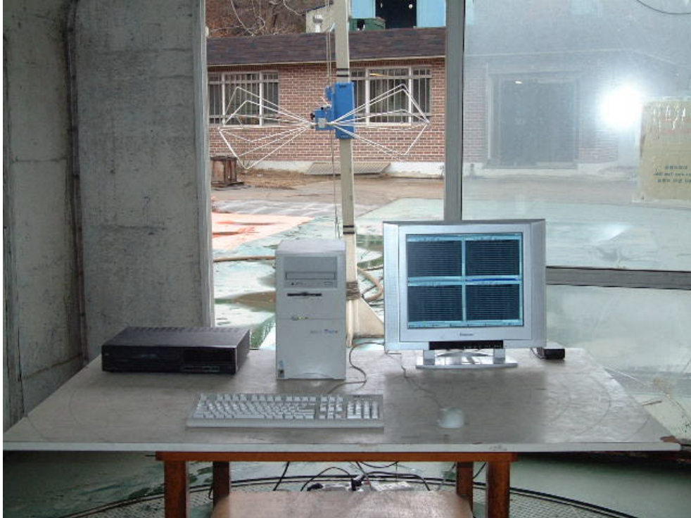
RADIATED EMISSION SETUP PHOTOGRAPH - FRONT VIEW ( 30 - 300 MHz )
