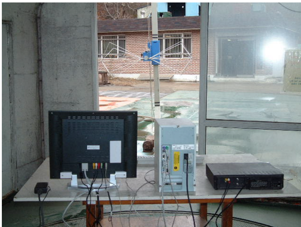
RADIATED EMISSION SETUP PHOTOGRAPH - REAR VIEW ( 30 - 300 MHz )
