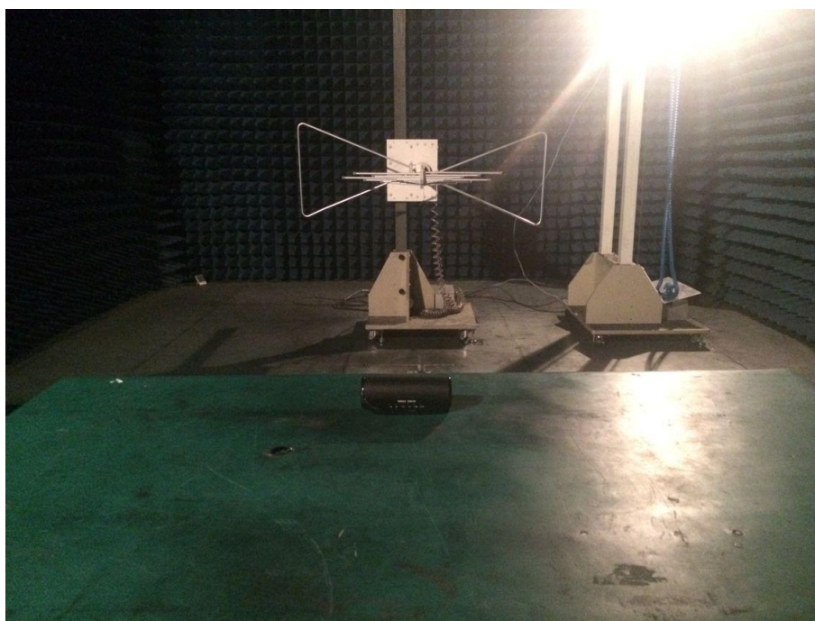
Radiated Emission test view (Frequency above 1GHz)
