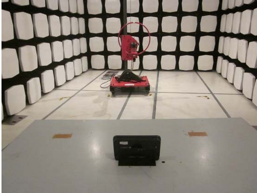
Measurement of Radiated Emission Test Set Up
