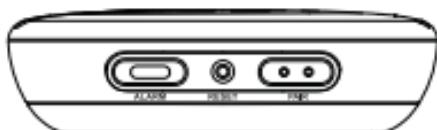
If the Vibration Alarm is not working properly, press RESET button to reset the unit. During reset, the LED flashes twice in (purple) color and the Vibration Alarm vibrates twice. Then the LED will flash once per 6 seconds in red color.
