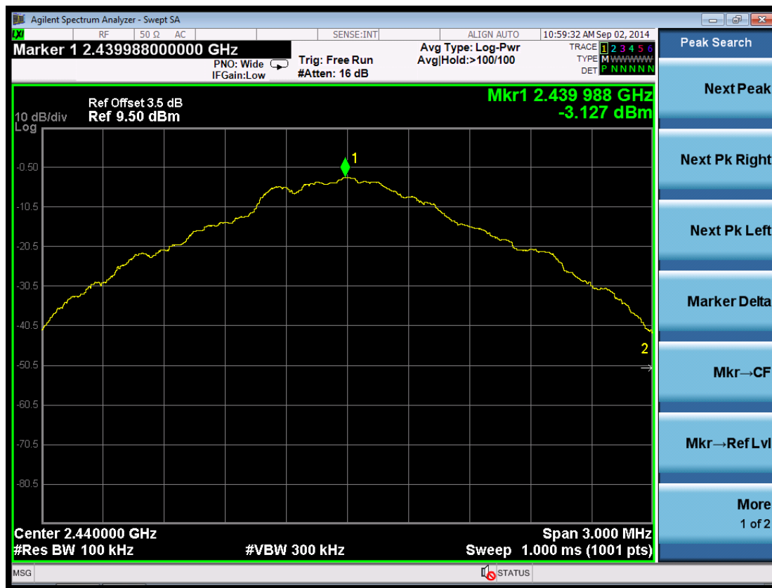
(Plot 6.6.1 B1: Channel 19: 2440MHz @ GFSK)
