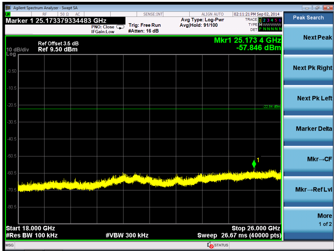
(Plot 6.6.1 C6: Channel 39: 2480MHz @ GFSK)
