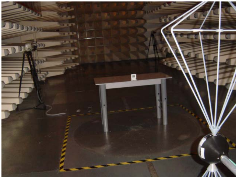
Set up of radiated emission test
