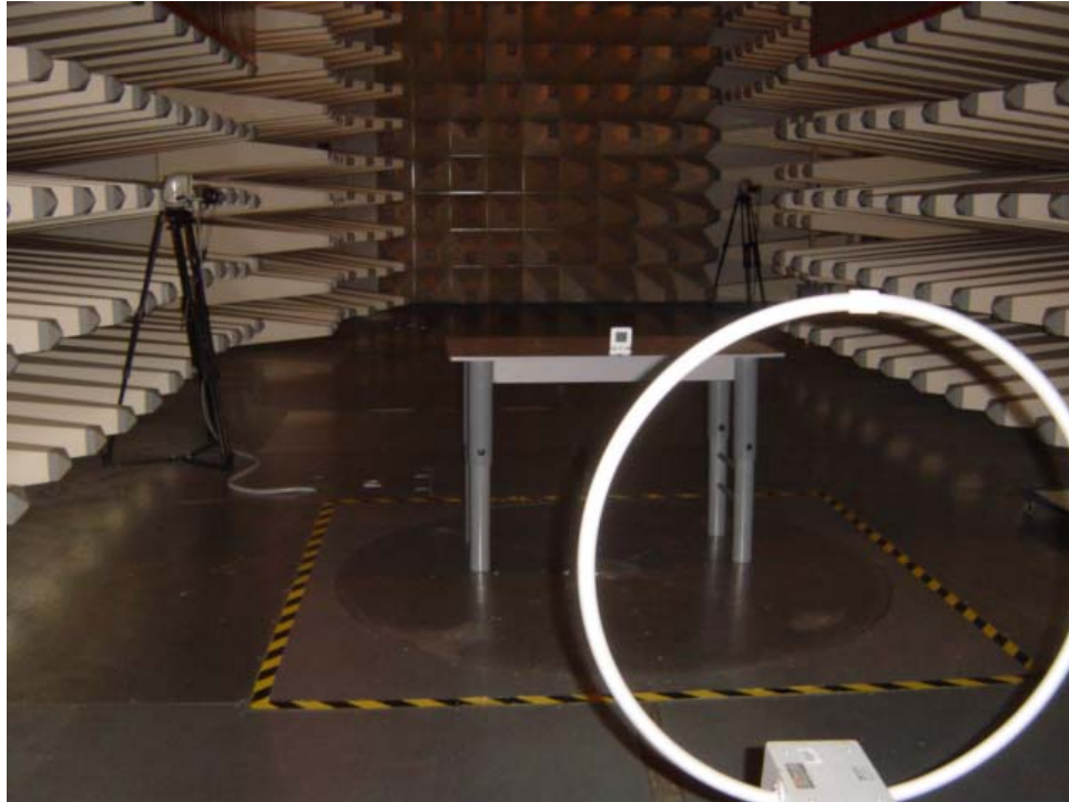
Set up of radiated emission test
